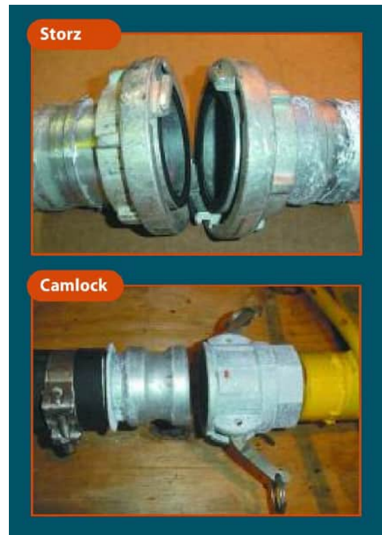
Example Storz and Camlock Couplings
